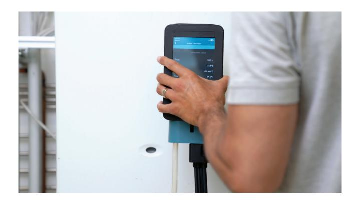
When performing a combustion analysis of the various combustion parameters, the user may often need also a pressure manometer, in order to simultaneously check and/or adjust gas pressures of the equipment. Thanks to the possibility of measuring combustion parameters and gas pressures at the same time, the newly developed Novo drastically reduces service time and limits the need to use different devices.
