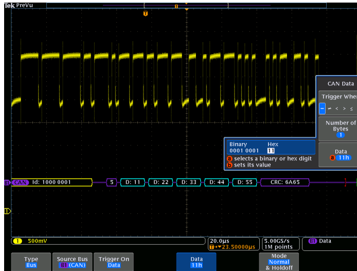
Figure 16: Triggering on a specific data value on the CAN bus.
