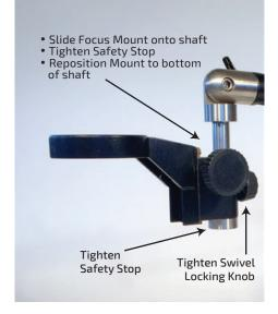
**6.** Slide Focus Mount onto Drop Arm shaft. Lightly tighten knob. Screw Safety Stop onto end of shaft firmly. Reposition Focusing Mount down to Safety Stop and tighten knob. Slide microscope head into Focus Mount opening and secure small locking knob.
