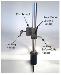
**2.** Position Safety Collar at approximate working distance. Tighten it's lock handles firmly. Insert locking handles into Articulating Arm locations shown and screw in several turns, but do not tighten.
