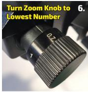
**NOTE:** For trinocular microscope models, keep the microscope body set to its **lowest zoom setting**, and twist the knurled rubber ring on the CCD adapter until what you see is in focus. Verify focus by zooming through the entire magnification range, and adjust slightly if required. This focus adjustment should not need to be completed again unless you remove the camera.
