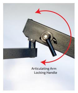
**4.** The angle adjustment of the Articulating Arm will be routinely secured by the Locking Handle. Loosen counter-clockwise to desired angle and tighten firmly.
