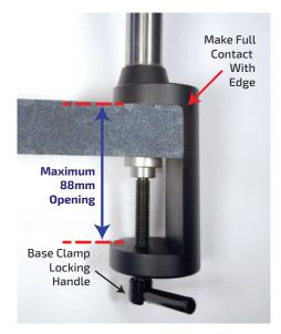
**1.** Screw Main Post into Base Clamp Base then Slide jaw of Base Clamp onto edge of table top. Ensure full contact of the clamp.
