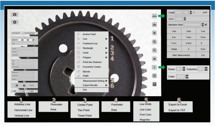
Each system ships with our exclusive **5MP Hybrid HDMI/USB Camera**. This exceptional smart camera pulls double duty for both production and quality assurance needs. It features both HDMI and USB outputs, and has integrated **smart camera controls** with a **host of onboard software features including**:
