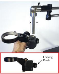
**5.** Slide microscope Focusing Mount up onto shaft. Tighten the Locking Knob lightly.
