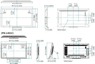
Units: inch (mm)  $^{*}$  To use the VESA-standard mounting bracket, use M6 screws that are 8 to 10 mm plus the thickness of the bracket.
