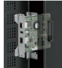
An optional board can slide into the slot on the back of the monitor.
