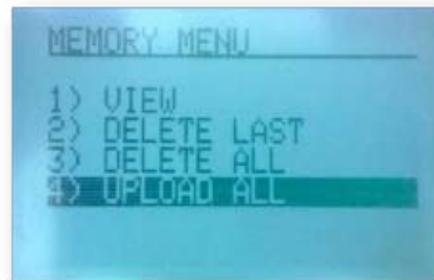
3. All memory stored on the instrument will immediately load on the table. Click on the Files menu at the top and select from the drop down box to save the data, print or export to Excel. If you are through with reviewing this data, click on New under the Files drop down menu to clear the screen. To open previously stored and saved data files, go to the Files menu and select Open from the drop down box.
