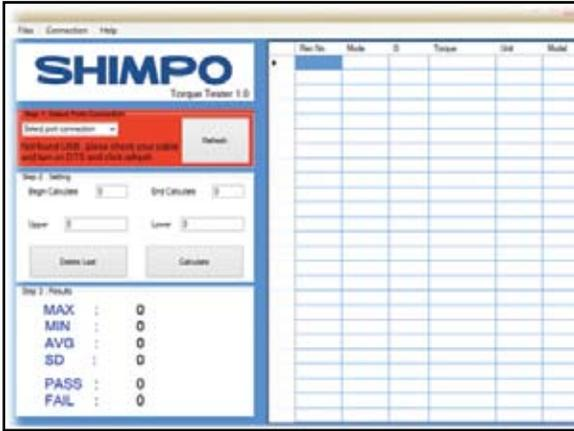
4. Once a connection is successfully made, the red box will change color to blue indicating the software is communicating with the TT unit and ready to use.
