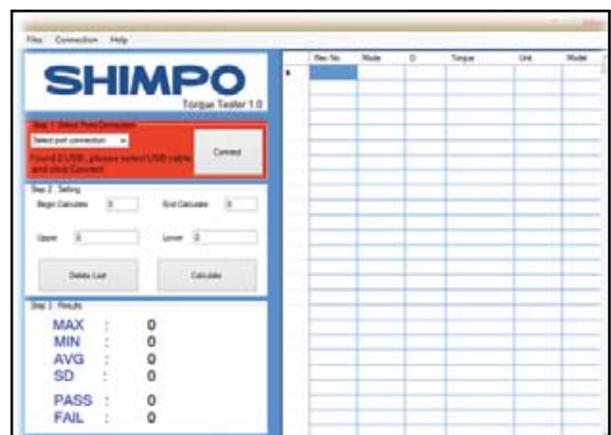
If the USB port is not found, you must check that the USB cable is not loose and is properly connected. Turn off the torque tester and then turn back on. Click the Refresh button.
