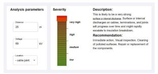
Recognize PD issues and determine severity with FLIR Severity Assessment, included in the
