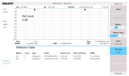
4) Connect the device under test with the DUT terminal of the reflection bridge. The cables or adapters between the DUT and bridge should as short as possible, in order to reduce extra mismatches. The resulting display appears as below. The trace on the screen is the return loss of the device under test.
