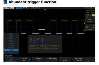
SDS1000X has a wealth of trigger modes, including Edge, Slope, Pulse, Video, Windows, Runt, Interval, Time out (Dropout), Pattern, IIC, SPI, UART/RS232, LIN, CAN
