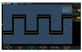
The SDS1000X utilizes a hardware-based Pass / Fail function, performing up to 60,000 Pass / Fail decisions each second. With easy to generate user-defined test templates, the SDS1000X compares the current measured trace to the template mask trace making it suitable for longterm signal monitoring or automated production line testing.
