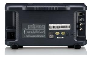
SDS1000X supports USB Host, USB Device (USBTMC), LAN (VXI-11), Pass/Fail and Trigger Out
