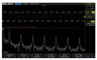
In addition to the traditional (+, -, \*, /) operation, SDS1000X oscilloscopes supports FFT, integration, differentiation, and square root operations
