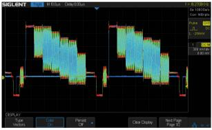
The color temperature display is similar to the intensity-graded trace except that the trace occurrence is represented by different colors (color "temperature") as opposed to changes in the intensity of one color. Red represents the most common occurrences or probabilities while blue are the least common points.
