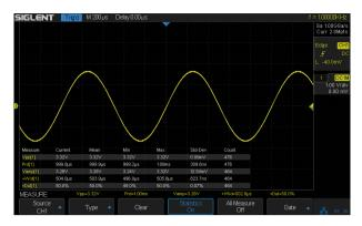
Parametric statistical functions to display any parameters of the five measurements: current, average, Minimum value, Maximum value, and the standard deviation. The measurement count is also displayed. The maximum number of parameters that can be measured and simultaneously analyzed statistically is five. Support Gating measurements, Math measurement, History measurement, Ref measurement.
