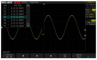
Playback history waveform to observe unusual events and locate the source quickly through the cursor or measurements, Located on the keyboard panel, this function is easily enabled.
