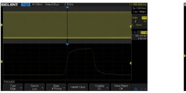
Using hardware-based Zoom technologies and record length of up to 14Mpts, users are able to use a higher sampling rate to capture more of the signal, and then quickly zoom in to focus on the area of interest
