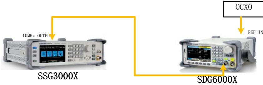
Figure 3-6 Connecting test instruments for frequency accuracy
