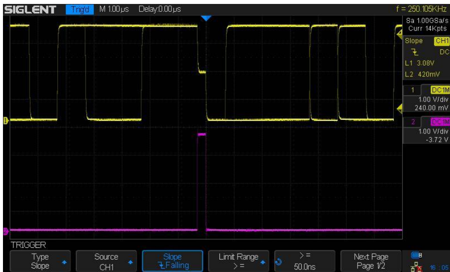
Figure 25 RUNT – Negative Edge Slope
