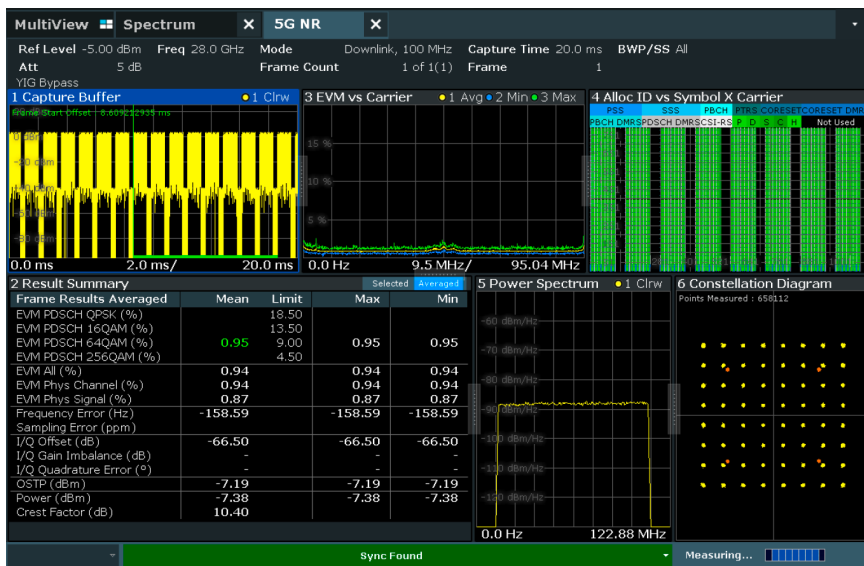
Analysis of a 5G NR downlink signal with R&S®FSW-K144.
