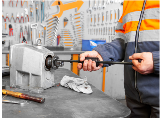
Knowhow: using a Seal Puller SP 50 to remove a radial seal from a gearbox without damage to the housing or shaft.
