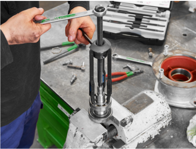
The Bearing Puller BP 61 enables ball bearings to be removed from shafts with ease and full control.
