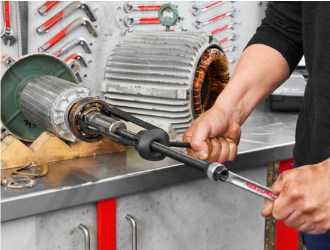
The Twin Puller TP 150 does it: a tightly seated bearing of an electric motor rotor is removed without risking damage to the housing or the shaft.
