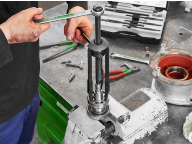
The Bearing Puller BP 61 enables ball bearings to be removed from shafts with ease and full control.
