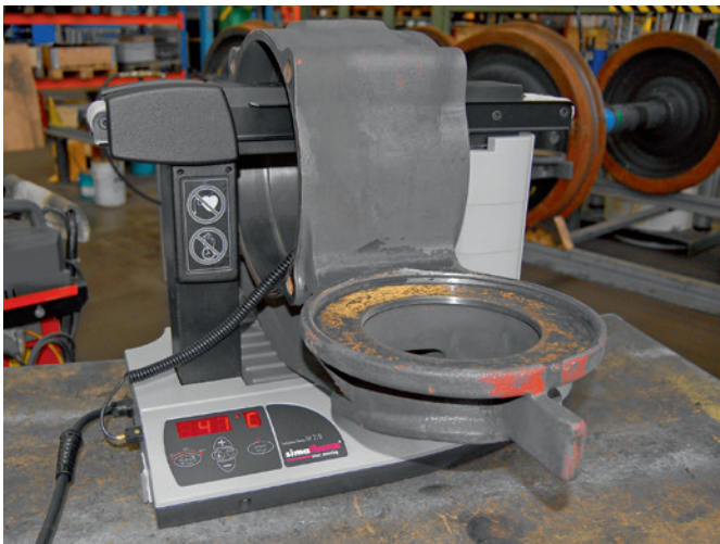
Working on a train wheel-set, the high-performance induction heater IH 210 heats a massive bearing housing to allow a bearing to be inserted.
