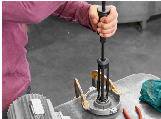
The Maintenance Kit MK 10-30 makes removing a ball bearing from an electric motor end cap straightforward.
