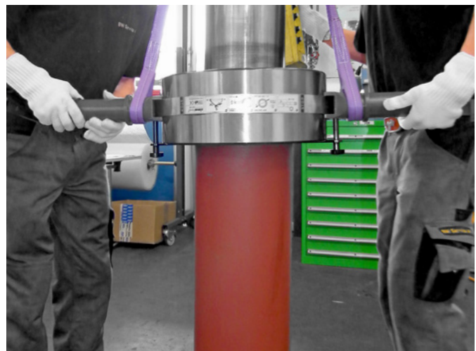
The Bearing Handling Tool BHT allows the heavy, pre-heated roller bearing to be safely lifted and accurately positioned on a turbine shaft.
