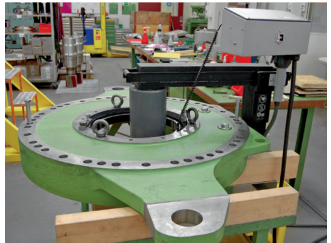
The largest and most efficient simatherm induction heater IH 240 is used here to heat the gearbox flange of a wind turbine.
