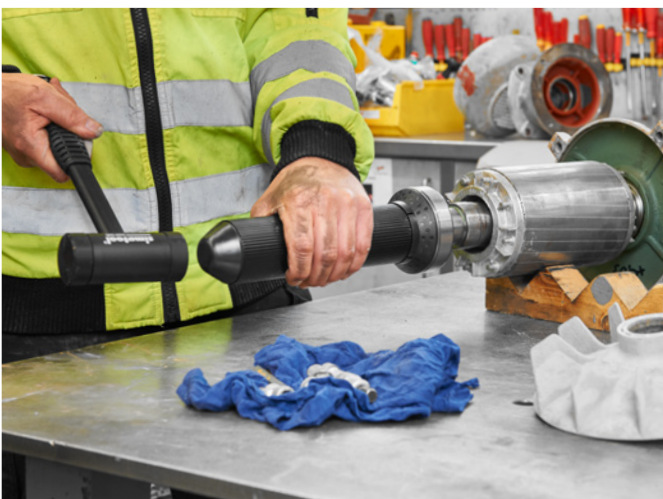
The Fitting Tool FT 33 ensures that the mounting force is evenly distributed across the inner and outer rings of the bearing and does not stress the rolling elements.
