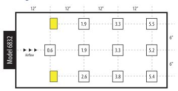
Discharge time in seconds (1000-100V), **fan speed set to high**; blower 12" from CPM measuring plate; CPM test plate 7.2" from table; discharge times slightly longer for 230 VAC, 50 Hz unit. Yellow cell without value = decay time over 30 seconds.
