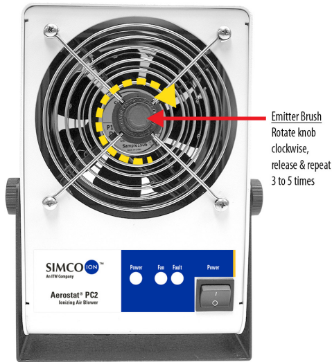
Figure 8. Manual Emitter Point Cleaning
