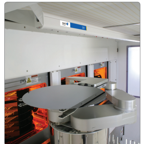
The industry-standard Digital AeroBar system provides balanced, optimized ionization inside tools and mini-environments.
