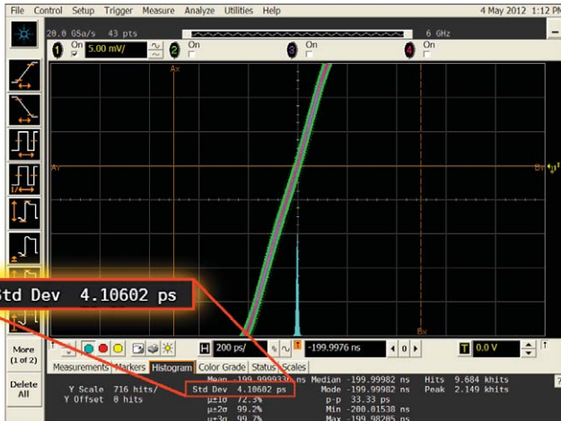
Figure 1. Jitter measurement on the 33522A waveform generator
