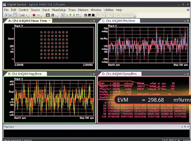
Figure 3. Constellation diagram and EVM of a 64-QAM baseband signal
