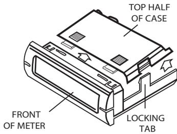
Using a screwdriver or thumbnail, spread the tabs on each side of the case to unlock the top half. Lift the rear of the top half and slide it away from the front of the meter.
