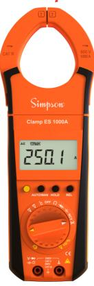
*Simpson Clamp ES* 1000/400*A* is a highly innovative design for features those increases safety and comfort of user. Continuity test, Temperature measurement (PT100/PT1000), overload warning, Auto off Cat II/III.
