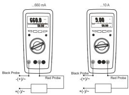
AC current measurement with(clip-on)current transformers
