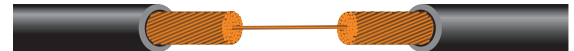
A Ground Continuity test could pass a product that has only 1 strand of wire connecting its chassis to ground.
