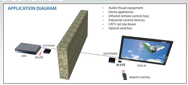
The IR-EYE is designed to work in combination with the IR-LED transmitter (sold separately). The IR-LED transmits the signal from the IR-EYE (via an infrared extender) to the media center device, so that an infrared remote control can be used to control it.
