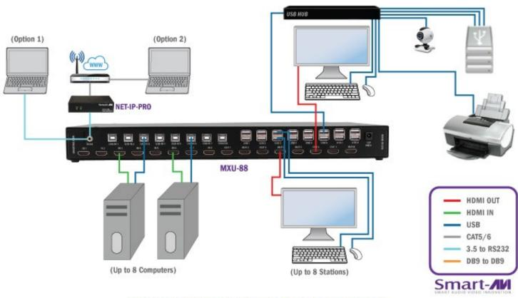
Transparent USB 2.0 Switching. Access to any USB Device for Any Station.
