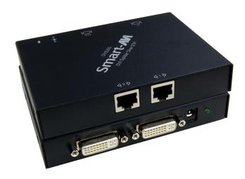
DVS-200 Extends Any DVI-D Signal up to 220 Feet toTwo Displays and One Local Screen Using CAT6 Cabling While Retaining Perfect Image Quality at Resolutions up to 1920 x 1200
