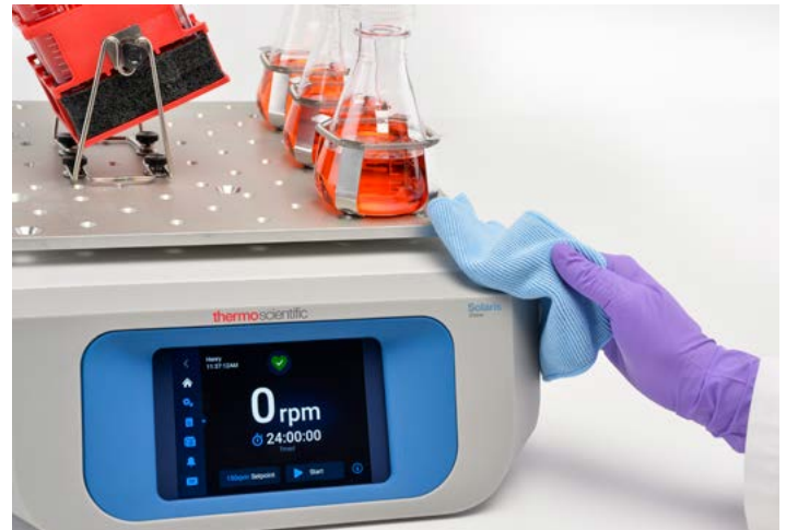
Figure 1: Rounded corners, clamps with one screw or less, removable platforms, sealed electronics systems and a touchscreen user interface all facilitate easy, frequent cleaning to prevent contamination.
