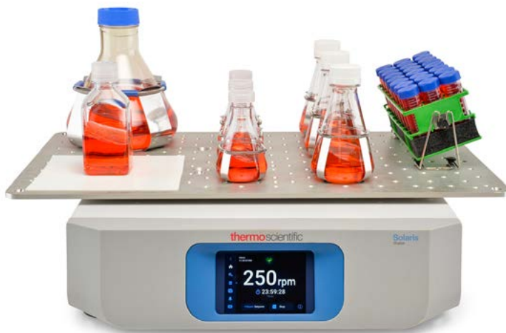
Figure 1: Different vessel types can be used on a shaker as long as they are balanced such that the weight is evenly distributed. If necessary, use a blank vessel as a counterbalance.
