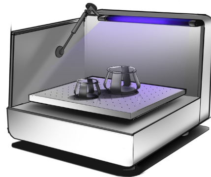
Figure 1: UV light is blocked by clamps, glass, plastic, etc. and will not decontaminate areas that it does not reach. The areas shown in shadow can continue to harbor microorganisms.
