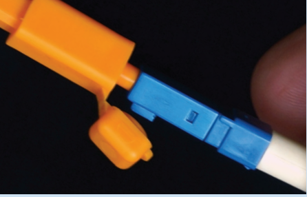
Flip open cap for cleaning connectors
