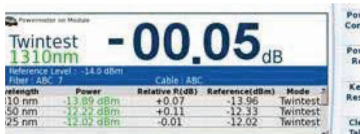
Fig. 48 Results and commands of the power meter
