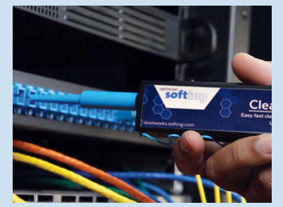
Remove cap for cleaning adapters and bulkheads
