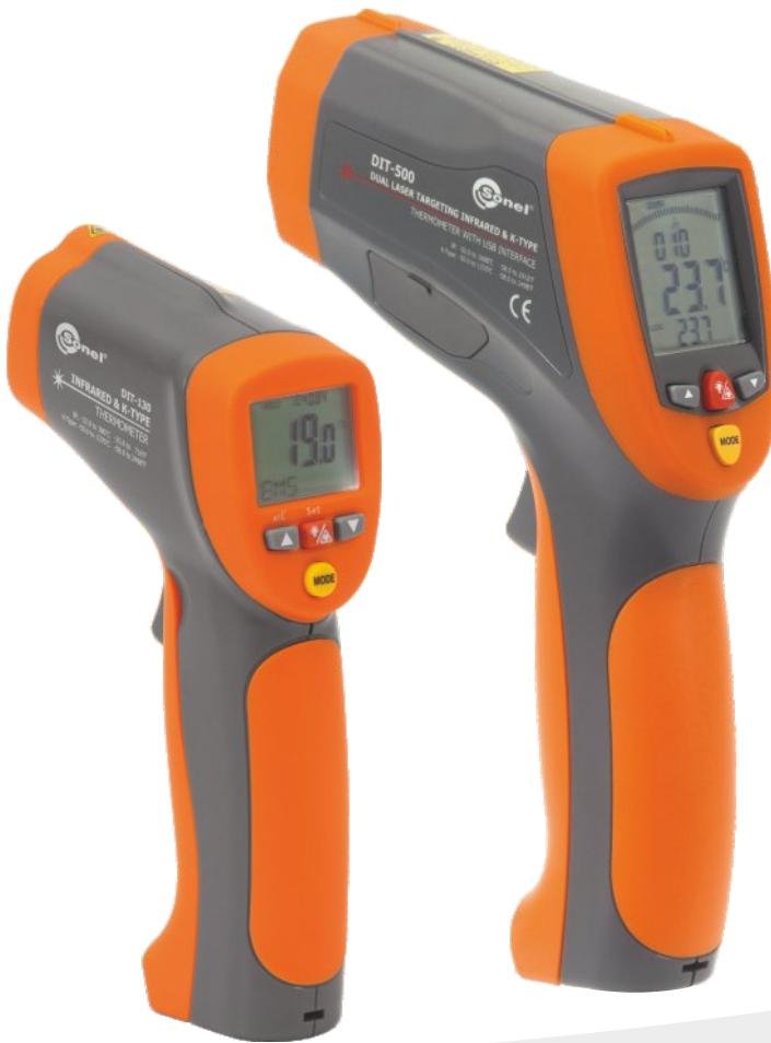
Temperature meters operating in the infrared are used to determine the temperature of the surface of the item. The optical system of the device detects the emitted, reflected and sent energy, which is collected and concentrated on the detector. Electronic system converts optical data into temperature value. In order to increase accuracy the laser pointer is builtin the device.
