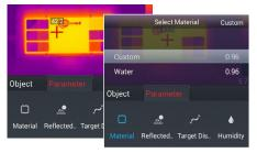
Select **Material** to change measured object's emissivity:
