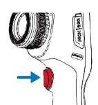
Press trigger to start/stop recording.
