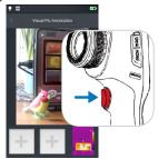
If you selected **Picture**, press the trigger button to take up to two photos in a visible light mode.
