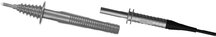
Fig. 39 Contact probe must be used with a blade probe or a crocodile clip.
