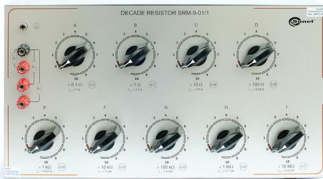
Resistance boxes of MC series are applied as reference standard equipment for verification and calibration of testers of electrical safety parameters of electric plants. The boxes parameters also enable to apply them for calibration of other types of widely spread electrical resistance meters.
