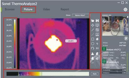
On the left side of the thermogram a temperature scale is shown with the colour corresponding to a given temperature.
