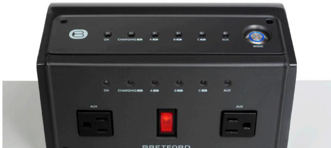
Power Management System regulates the power allowing all 30 computers to charge from a single outlet without the use of a timer.
