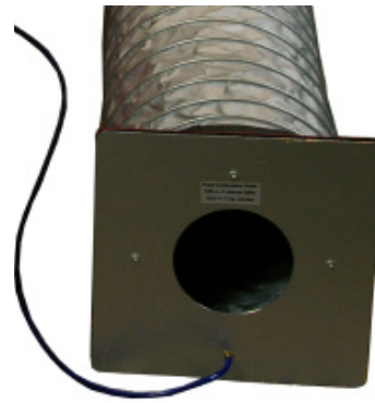
Field Calibration Plate verifies system in working condition. #DU159
