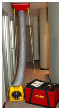
Pressure Pan Hood connects to ducts for leakage and flow measurement. #PP105
