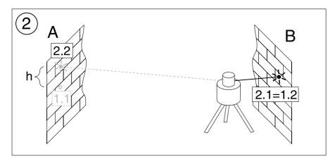
If the unit is within its working accuracy limits ( $\pm$  20") the maximum difference from true level at 20 m (65 ft.) + 20 m (65 ft.) = 40 m (130 ft.) is 4 mm (3/16 inch).
