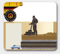
LINE ALERT: This unique feature is ideal for working in high-vibration or wet conditions where the pipe lasers may be disturbed. The beam flashes to notify you that the setup line has been disturbed, eliminating the necessity of rework. Combined with the self-leveling warning, you'll always complete the job correctly, on time and on budget! Only available on the DG711.
