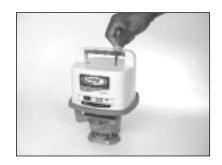
**Note:** The laser has reverse-polarity protection. If the batteries are put in wrong, no damage occurs to the laser but it does not work. Allow it one minute to recover after the batteries have been installed correctly.
