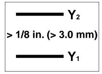
To correct for a calibration error, position the receiver at the midpoint of the two elevation marks on the wall.
