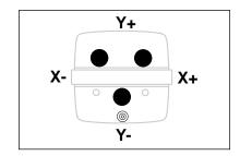
**Note:** Left-thumb rule—both thumbs in, both thumbs out, the bubble follows the left thumb.
