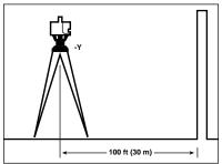
Raise/lower the receiver until you get an on-grade reading for the -Y axis.
