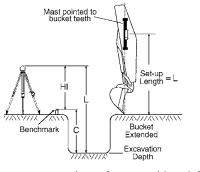
1. Set the laser up in an appropriate location for receiver visibility and efficient machine operation and turn it on.
