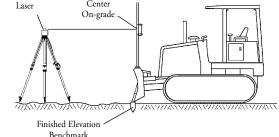
1. Position the machine so the blade can be set to the desired finished elevation (typically on a benchmark or hub stake)
