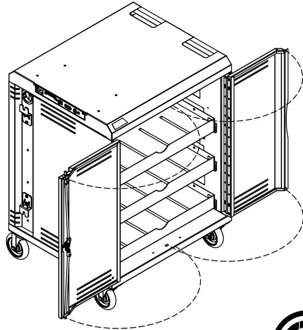
Use the VR Cart to store, transport, and charge up to 30 virtual reality devices. Protective foam on a pull-out tray protect and provide easy access to the devices. The cart's compact footprint and top handles provide easy mobility. Locking doors and panel increase security. This economical cart is made with heavy-gauge steel for security and powder-coated for a durable, long-lasting finish.
