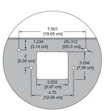
Mounting holes and cutouts needed on flat end of worksurface
