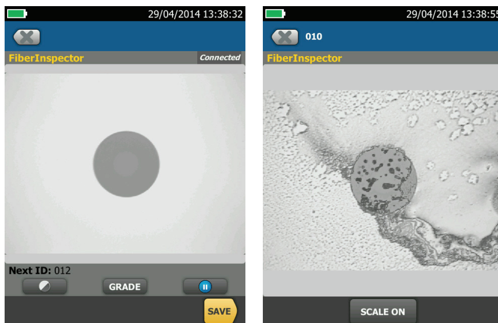
Figure 5: Specialized solvents (left) are far more effective at cleaning end-faces than IPA that can leave behind a residue (right).
