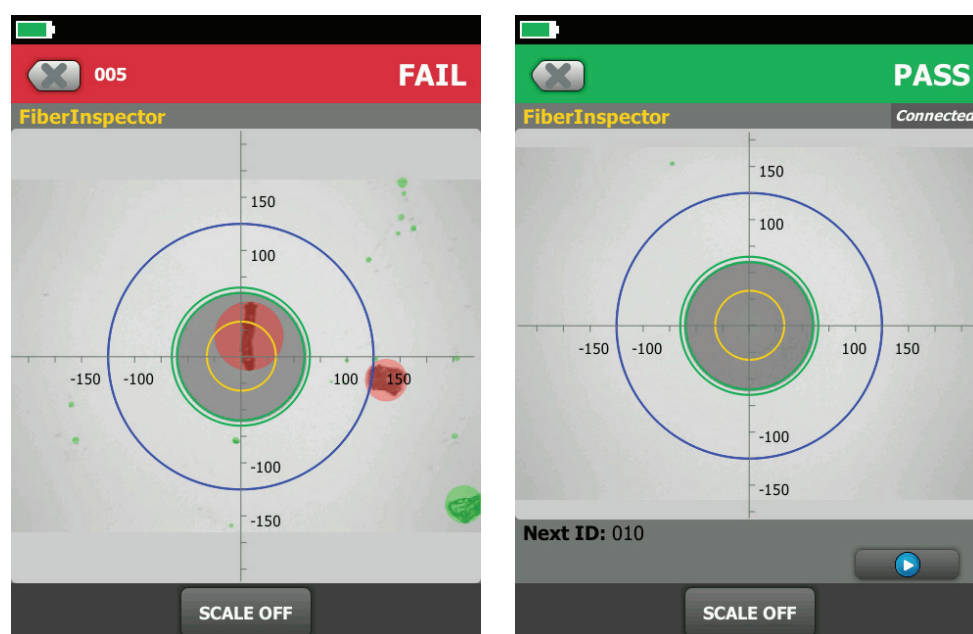
Figure 6: The FI-7000's certification results allow you to quickly determine if the fiber end-face pass or fails. An example of a failing end-face is shown on the left and a passing end-face is shown on the right.
