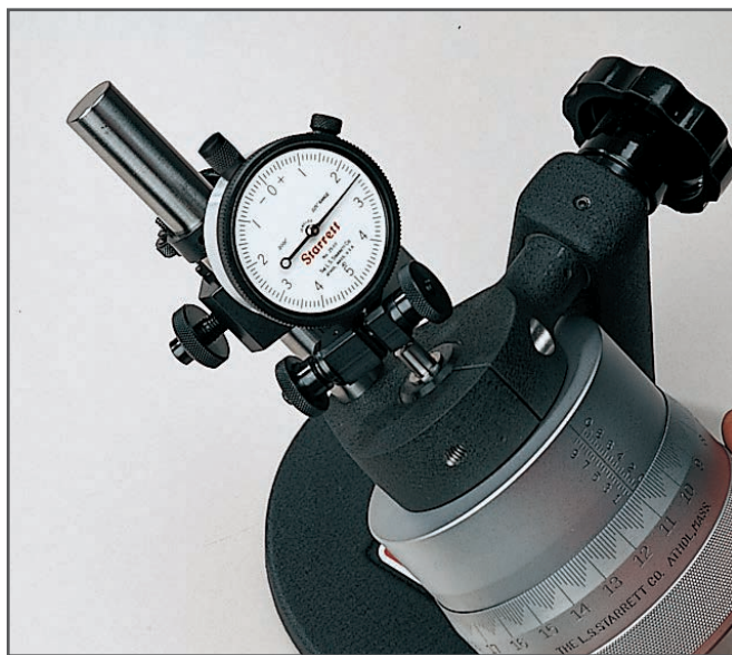
Checking AGD dial indicator
