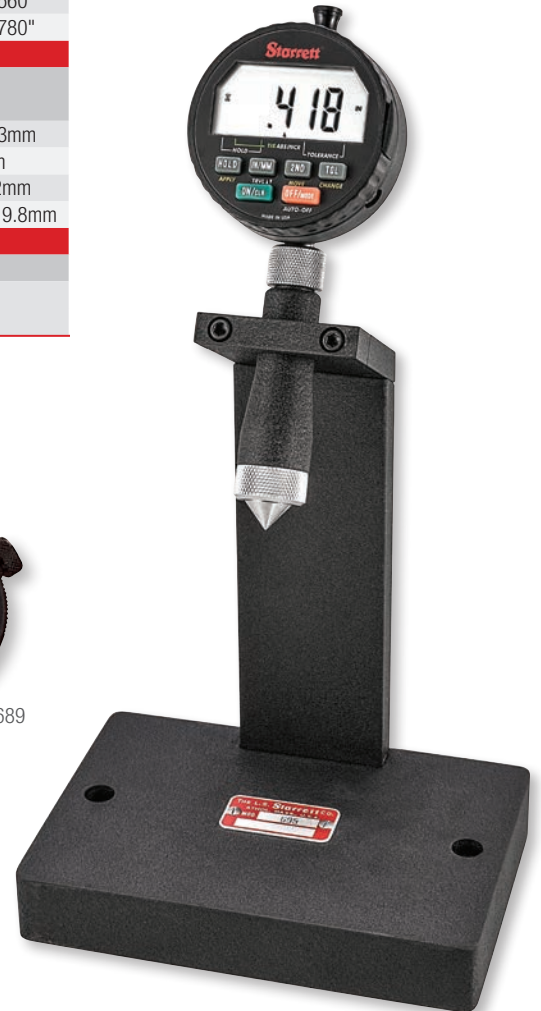
687-3Z Countersink Gage with 695 Check Stand with F2720-41Q Electronic Indicator
