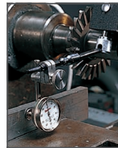
657A with 196B1 Universal Dial Indicator setting up workpiece on milling machine.
