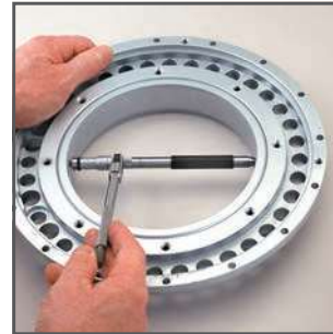
Rods attachable as shown to either one or both ends of the head ensures the best balance, feel, and ease of reading.
