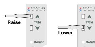
4.0 Once trim is complete allow 30 seconds with no button press, the transmitter will time out and return to normal operation.
