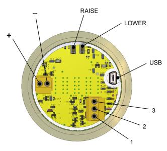
A – In order to setup the SEM710 connect a USB port on your computer to the USB port on the SEM710 using a USB type-A / Mini USB 4-pin cable. Start the Status Instruments USB LINK Software and setup the temperature range that you want the 4 to 20mA output to be. Also make sure the TRIM feature is turned on.
