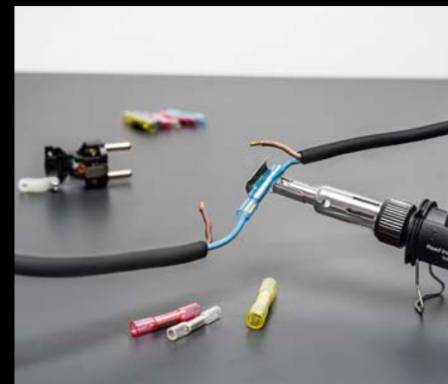
Create an even seal on solder sleeves
